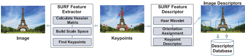
Fig. 5. Image matching pipeline.
